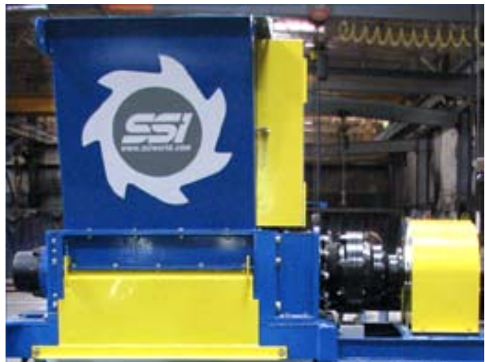
The SR-300 features a direct drive design (no belts) and a magnetic clutch for shock protection.
