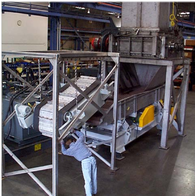
SSI shredder integrated with secondary processing equipment to deliver optimal system performance
