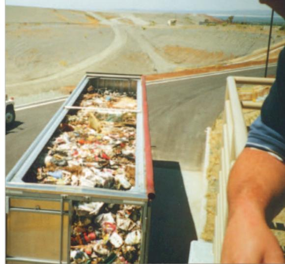
Constant density 25-ton payload in trailer (Top cover removed for photo)
