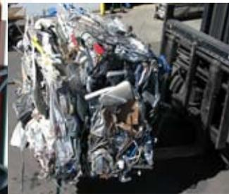
***Scrap compactor processing white goods. 30 TPH rate with 4:1 reduction ratio!***
